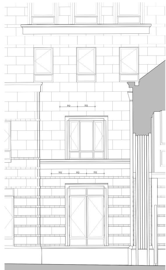
Above: brick and stone coursing for a corridor between the twin midrises (Revit)
